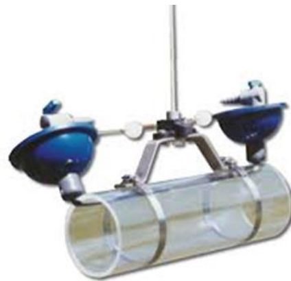
Figure 4. Labelled diagram (top) and photograph (bottom) of the Van Dorn Sampling Bottle.
