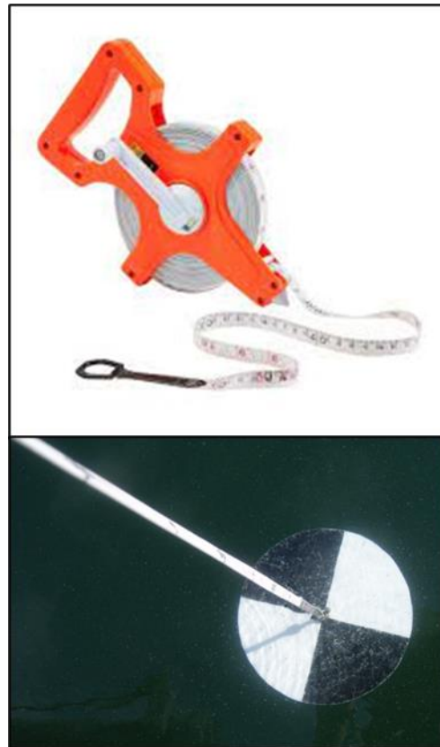
Figure 3. Top - Field tape to measure maximum depth at the site. Bottom – Secchi disk being lowered down the water column.
